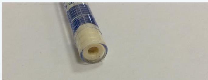
In the past stoppers were sealed with paraffin in order to produce an airtight seal against the glass walls of the cartridge. Glycerin was added into the channels around the stopper as a lubricant, allowing it to slide into the glass cylinder more easily. Today, most plungers are siliconized thus eliminating the need of both the paraffin and the glycerin. As a matter of fact, “Sticky stoppers” (stoppers that do not move smoothly down the glass cartridge) are infrequent today.
