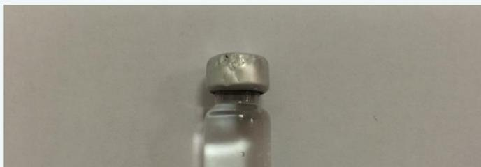
**Actions:** *in the case of a damaged cap, discard the cartridge and inform the manufacturer of the issue providing full details of the complaint (lot number, defect description, etc.)*
