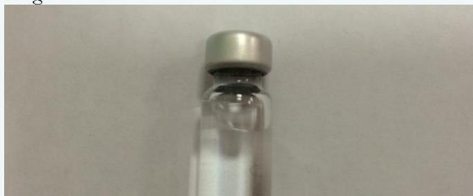
**Actions:** *shake the cartridge and place it vertically with the cap uppermost. Bubbles should disappear in the neck; if not, then the bubble is too large and the cartridge must not be used. Discard the cartridge and inform the manufacturer.*
