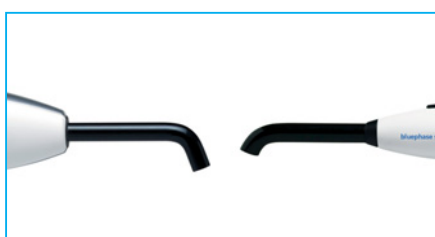
Fig. 9: Access to the treatment site is improved due to the shortened light probe of bluephase style.
