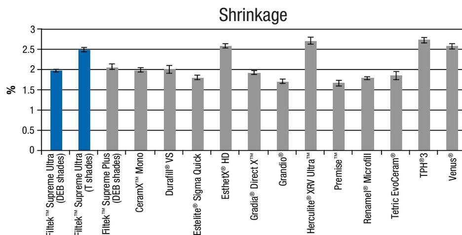
The volumetric shrinkage of Filtek™ Supreme Ultra Universal Restorative DEB shades and T shades is statistically different. The DEB shades of Filtek Supreme Ultra restorative are statistically lower than EsthetX HD, Herculite XRV Ultra, TPH3 and Venus.
