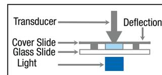
In this test, samples were exposed for 60 seconds to a 3M™ ESPE™ Visilux™ 2 Visible Light Curing Unit. The final shrinkage was recorded 4 minutes after the end of light exposure.
