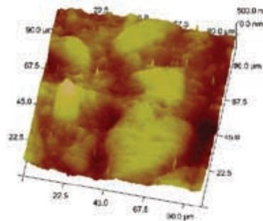
The AFM<sup>11</sup> (Figure 7) is a 3-D image of the surface of a microfill after 6000 cycles of toothbrush abrasion. Microfills have proven to retain their polish (surface reflectivity) over time. The prepolymerized filler particles are marginally more wear resistant than the surrounding matrix, resulting in small surface irregularities.
