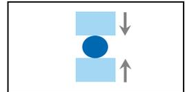
The diametral tensile strength of Filtek Supreme Ultra restorative is comparable to Filtek Supreme Plus restorative. The diametral tensile strength is statistically significantly higher than the microfills Durafill VS and Renamel Microfill. In addition, it is statistically higher than CeramX Mono, Estelite Sigma Quick, EsthetX HD, Gradia Direct X, Premise, Tetric EvoCeram, TPH3 and Venus universal restoratives.
