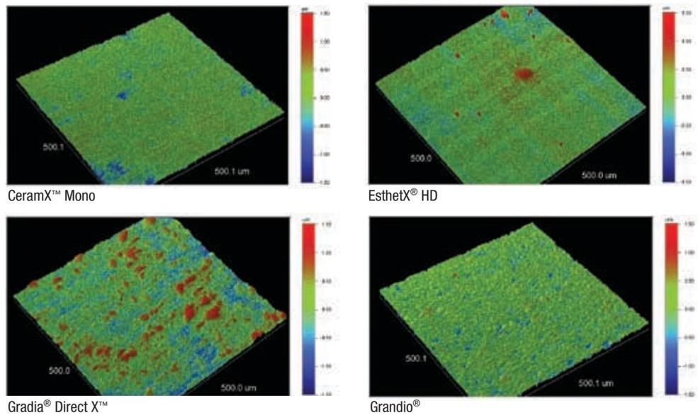
Gradia Direct X exhibits a very rough surface after toothbrush abrasions. (Ra~287 nm) The Wyko image shows orange protrusions and deep blue valleys in the surface. The Grandio surface shows a smaller peak-to-valley ratio (Ra~226 nm) than Gradia Direct X, but is still very rough (the color across the sample is not uniform).
