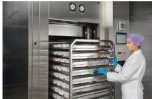
In the terminal sterilization process, the product must be treated with a high temperature autoclave process (at least 121°C) to kill eventual microorganisms inside. The dead bacteria will stay inside the cartridge or vial.
