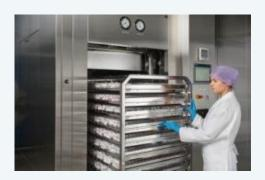
In Terminal sterilization process, the product must be treated with high temperature autoclave process (at least 121°C) to kill eventual microorganism inside. The dead bacteria will stay inside the cartridge or vial.
