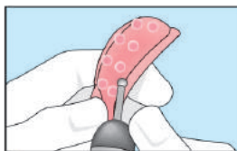
3 Remove resin with round bur for thickness of lining
