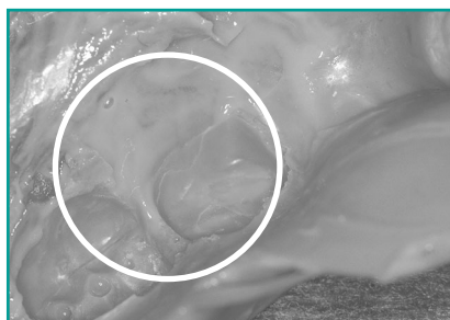
“Streaky” inadequate mix
